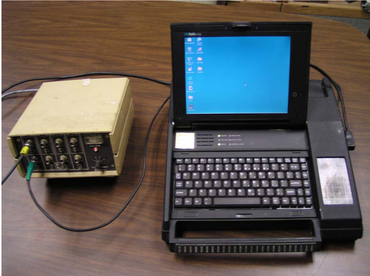
Figure 6. Setup for collecting data from microphone sensor
